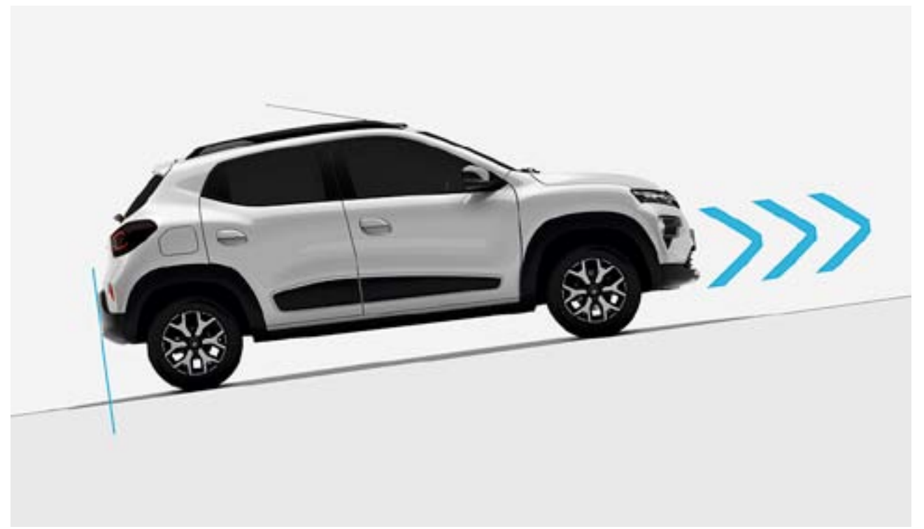
hill start assist Hill Start Assist (HSA) keeps the vehicle stationary on slopes, giving you time to start safely without rolling backwards.
