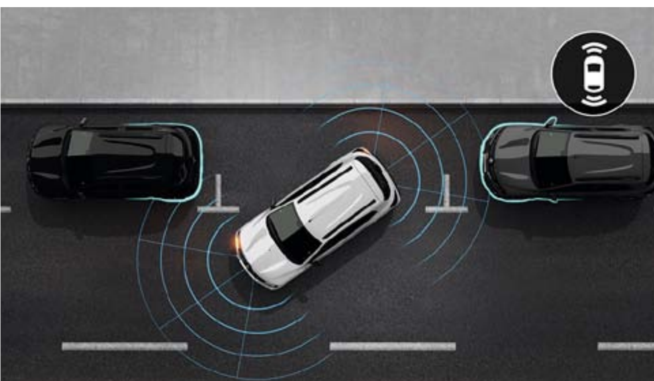
parking sensor The parking sensor emits an audible alert when an object is close to the vehicle, offering greater safety during manoeuvres.
